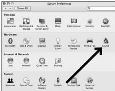
4. Click the **Input** tab and select the **AT2020USB+** as the device for sound input.
