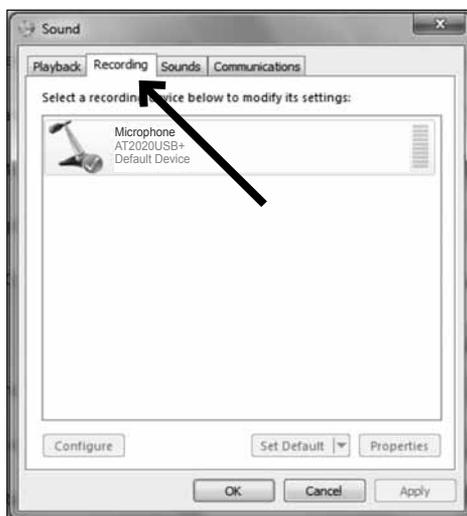
7. Double click on the AT2020USB+ icon to open the **Microphone Properties** window. Select the **Levels** tab to adjust microphone level (loudness). You may need to come back to this window to readjust the level after you begin recording.
