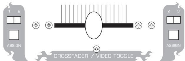
Note: If you assign channel 2 on both sides, the crossfader will not crossfade.
