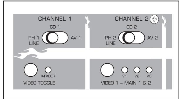
2. Press the VIDEO 1 button until the correct AV channel LED is lit.
