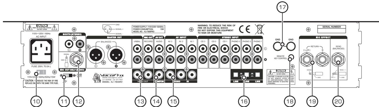
10. **VOLTAGE SELECTOR** - This switch can change the voltage from 115V to 230V. Before your KJ-7808RV is shipped from the factory, the switch is set to 115V. If you live in an area that has different voltage requirements (230-240V), you **MUST** set it to 230V.
