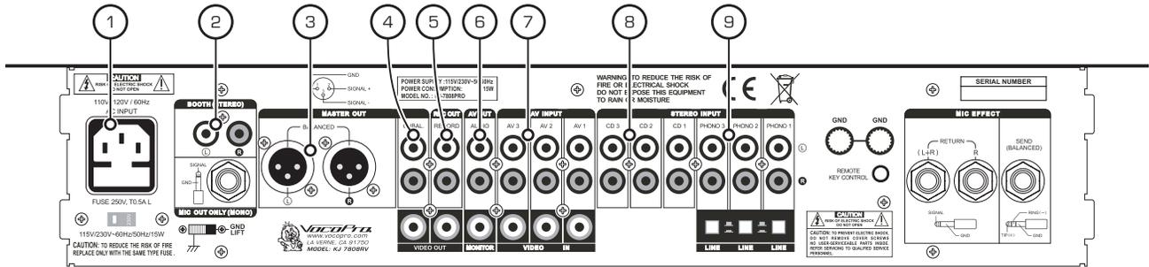
1. **AC INPUT** - This is the terminal for the AC power cable. Carefully insert the AC power cable here. The AC power cable should fit firm into housing.
