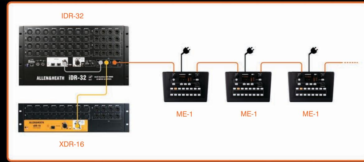
ME-1 can be connected to an ACE card fitted in Port B of an iLive MixRack.
