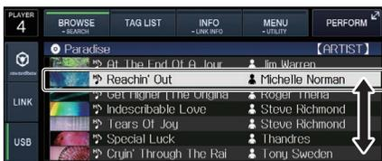
The jump function can be used by pressing the rotary selector for over 1 second.
