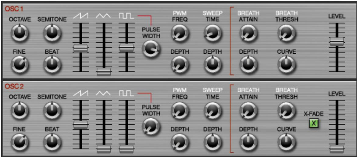
The EWI4000s has two analog modeled oscillators, which are editable independent of each other. Each oscillator outputs Sawtooth, Triangle and Pulse waves and includes a waveform mixer that lets you set how much of each wave is heard.
