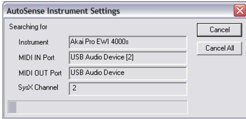
If the AutoSense procedure cannot detect your instrument's settings, you will need to make sure your Midi Interface drivers are installed correctly and that all cables are connected as per the diagram in Step 2. Make sure the output of your computer is connected to the input of the EWI 4000s (and vice-versa). Also ensure that no SysEx filtering is enabled on your MIDI interface.
