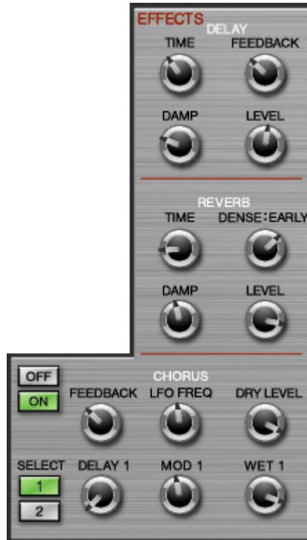
The EFFECTS SECTION consists of high quality chorus, delay, and reverb effects connected in serial:
