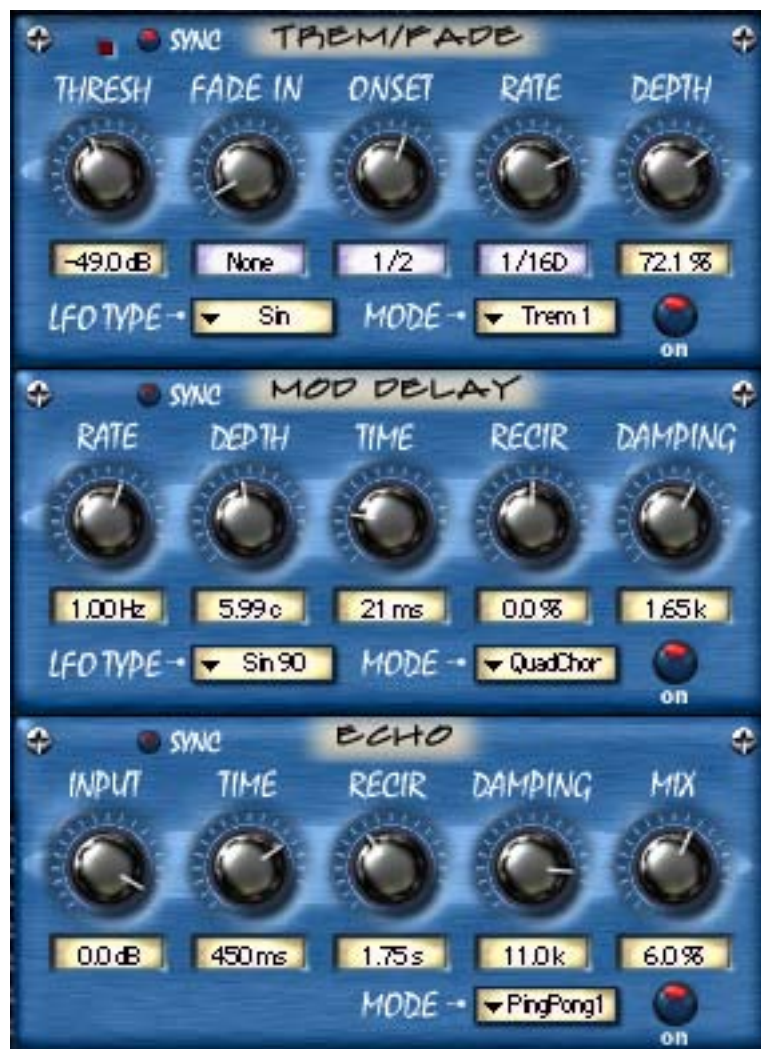
Figure 123. The TremModEcho plug-in contains three modules
