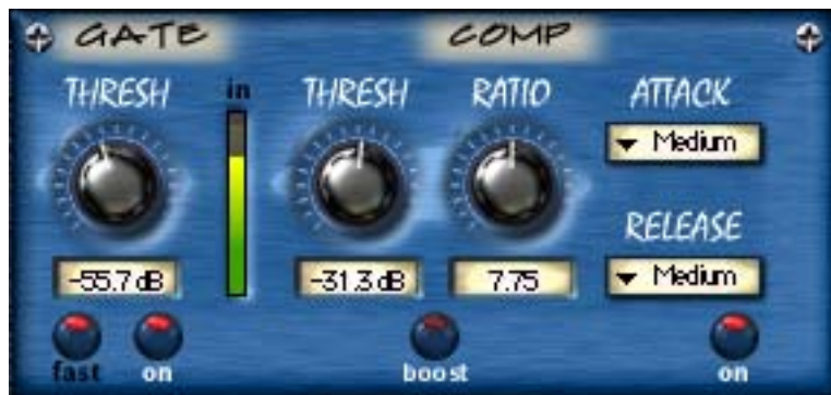
Figure 118. The Gate/Comp module
