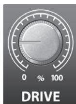
**Drive control.** The Drive knob controls the signal level being routed through the 12AX7 vacuum tube. The effect ranges from subtle to extreme, depending on the setting; the more signal being sent to the tube, the more distortion you will hear. This is great for guitar, bass, and even vocals, if that is the effect you want to achieve. Of course, in some applications, tube drive is not needed.
