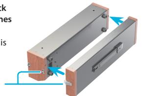
3. Using the stacking screws that you removed in step 1, fasten the two SYR-E84 units together.
