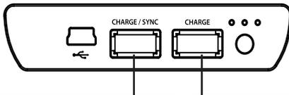
This output is compatible with most smart devices, but is only compatible with certain iPod models when the xeMini is also connected to a computer or external iPod charger, like the xePico.
