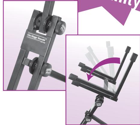
*Solid steel double stamped 3" disks allows for a secure locking position and customized angle adjustments, while the folding support arms saves space for storage and travel.*
