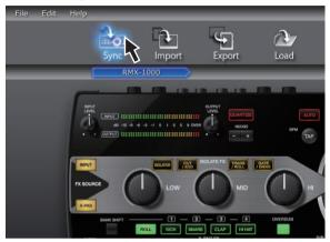
The customized parameter data is loaded onto the RMX-1000. After loading, [Syc] appears on the RMX-1000's BPM display section. The loaded customized parameter data can be checked when the RMX-1000's [SETTING] selector switch is set to the [USER] side.
