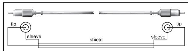
Fig. 4.4: RCA cable (for CD IN/AUX IN connection)
