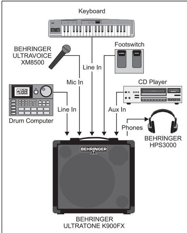
Fig. 3.1: Example of a setup using the ULTRATONE
