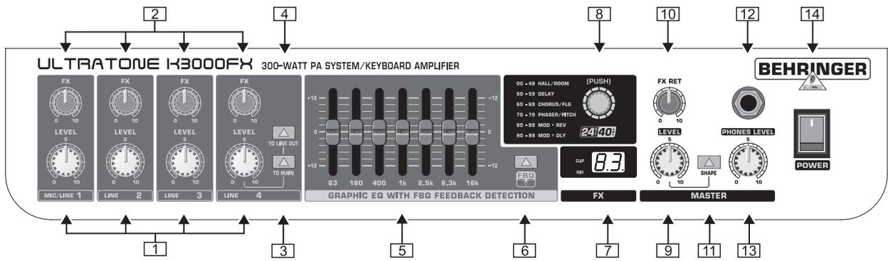
Fig. 2.1: Front panel control elements (K3000FX and K1800FX)
