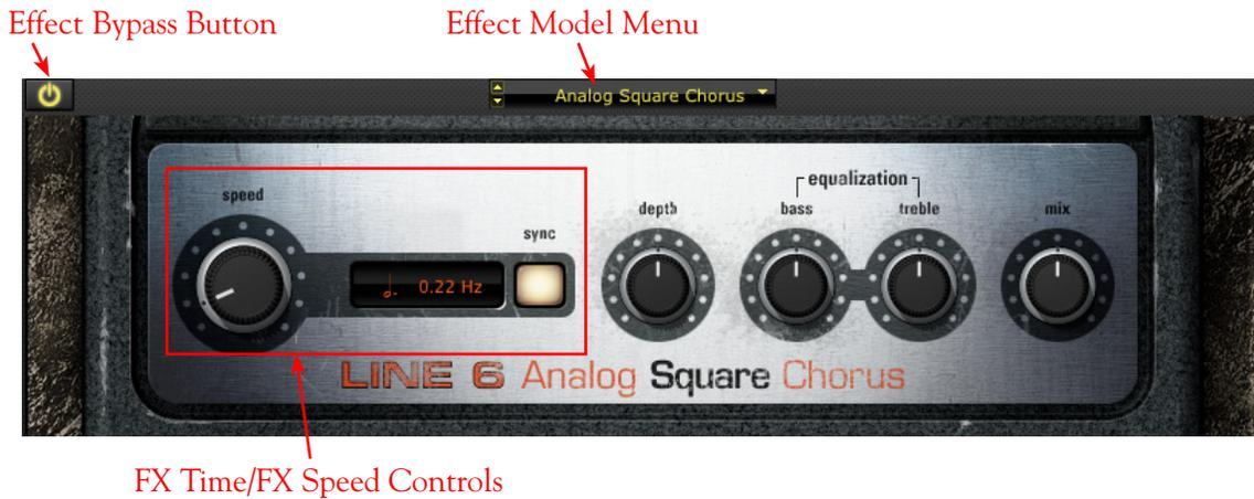
**Effect Bypass Button** - Bypasses the effect without removing it from the signal path
