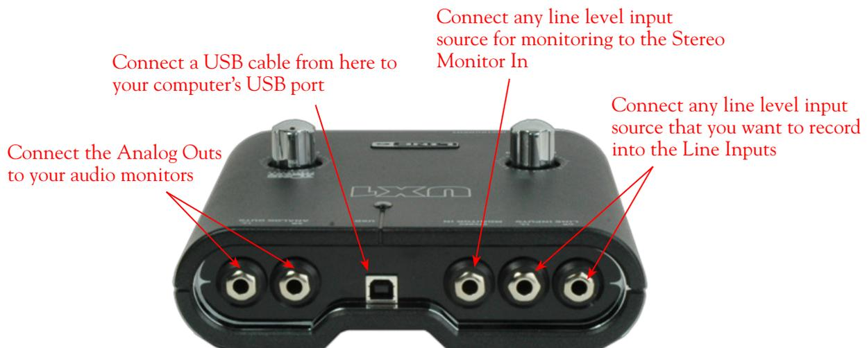
**Line Inputs** - To record the signal from a line level source, such as a keyboard, your stereo receiver, the line out from a mixing console, etc., connect them to these Left and Right inputs.
