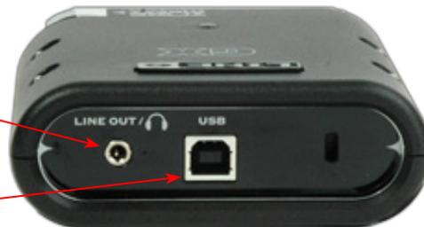
**USB** - This is where you connect the USB cable from GX directly to your computer’s USB 1.1 or 2.0 port.
