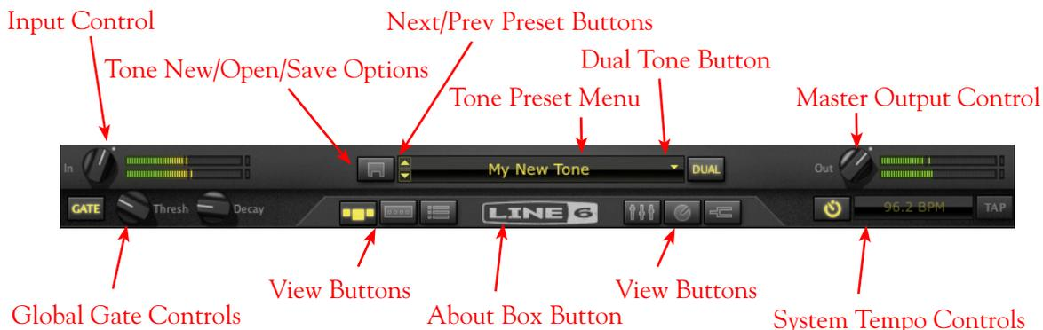
**Input Control** - Use the knob and meters here to optimize the audio signal fed into the Plug-In.\*
