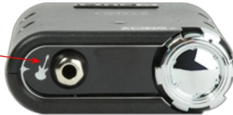
**Instrument Input** - Plug in your electric guitar or bass here to feed the instrument’s signal into the POD Farm 2 standalone application. This allows you to choose your Tone, and then route the processed signal to the Record Sends (to your audio software) and your ToneDirect™ monitoring signal directly to the hardware outputs.
