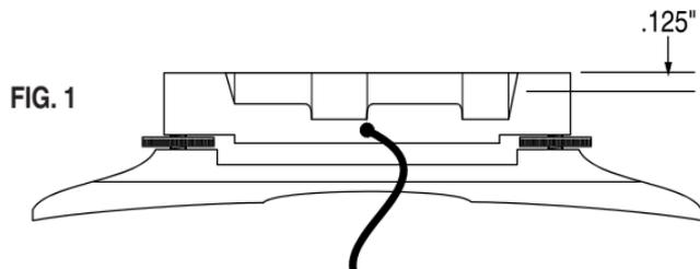
3. Remove the screw at the bottom of the tailpiece and replace with the supplied screw, washer and jack/clamp assembly. Fasten the assembly securely.
