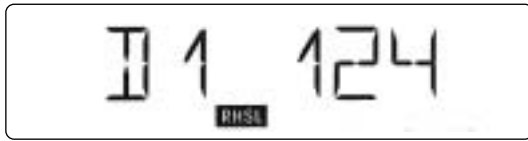
Example 1: Dropout no. 1 occurred after 124 seconds.
