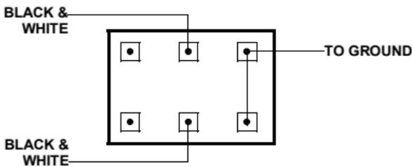
Again, the **GREEN** and **BARE** wires from both pickups go to ground. The **RED** wires on both pickup are the hot outputs.
