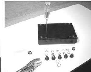
Knobs off, nuts & washers off, side jack nuts & washers off, now remove screws.
