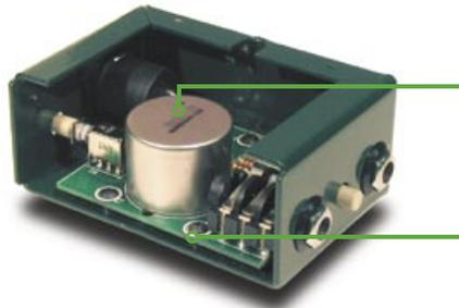
**HIGH PERFORMANCE** transformer for distortion-free signal transfer and 100% isolation from ground loop hum.
