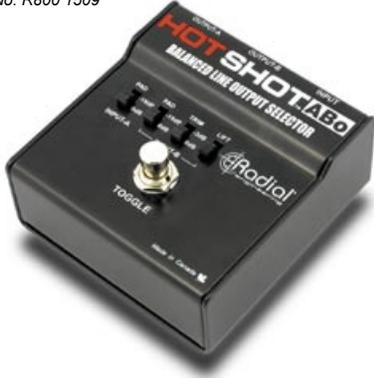
The Hot Shot ABo is a balanced line selecting device that toggles a signal between two destinations. It features 100% passive operation with latching footswitch and therefore does not require any type of powering whatsoever. To add versatility both outputs are equipped with a -15dB pad and output B is equipped with a secondary -6dB trim to reduce the output going to a more sensitive source.
