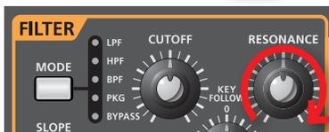
**5.** Slowly turn the FILTER [CUTOFF] knob from the maximum position down to the minimum.
