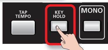
4. Press and hold any key. The wind will start blowing.
