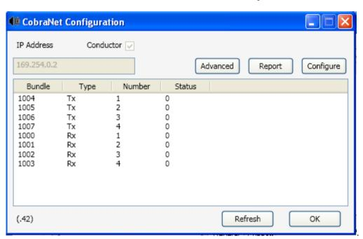
5. The bundle numbers can now be changed as required by either directly editing the bundle number fields, or selecting one of the four transmit or receive bundles and clicking the 'Configure' button, which opens a more detailed Configuration dialogue box:
