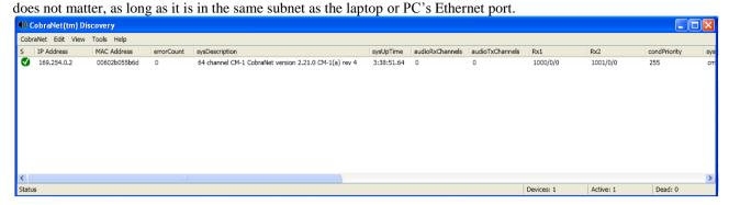
4. To configure the Cobra $Net^{TM}$  card right-click on the Si Cobra $Net^{TM}$  device to select it, then choose **Tools>Configure**.
