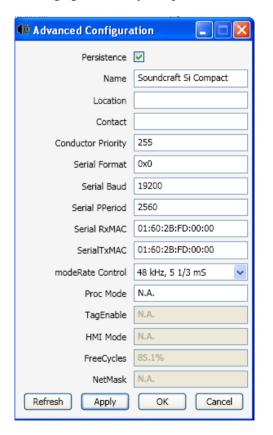
The Advanced Configuration dialogue box is used to set the Latency and Sample rate of the Si CobraNet<sup>TM</sup> card (this is the parameter called **modeRate Control**)
