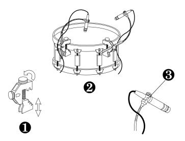
**WARNING:** Do NOT tighten the thumbscrew on the plastic section of the connector as this could cause damage. **NOTE:** To minimize potential noise or damage, position the microphone outside the drummer's range of stick movement and cymbal movement.
