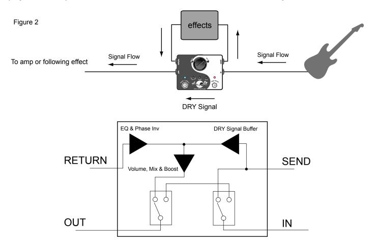
**Volume** adjusts the main output only when the blend switch is activated. As the above diagram shows, the volume affect both the direct and effect signal.
