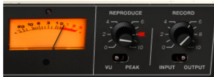
Figure 3. One side of the Ampex ATR-102 “penthouse” showing meter and I/O controls
