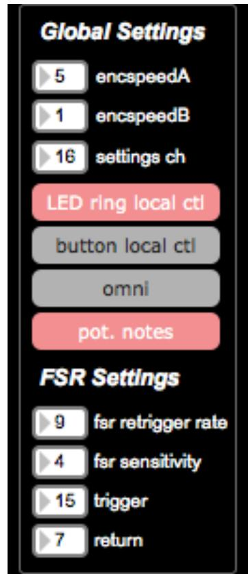
any channel settings of the incoming message and respond accordingly. For example, suppose the TWEAKER's bottom left button is configured to respond to note 37 on channel 1. If *omni* is off, then the TWEAKER would ignore any note 37 (on or off) received on any other channel. If *omni* is on, then that same note message would actually turn the LED on and off in response!
