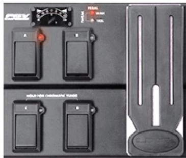
The FBV Express and FBV Express MK II will also control many Spider Valve MkII functions such as Tuner, Preset Select, Tap Tempo, and a few FX assignments for the pedal.
