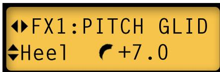
For example, with Heel at +7 and POS at 0, you get a 5th note, which is 7 half steps up.
