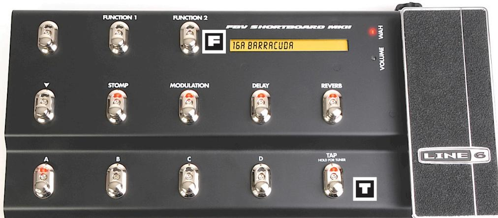
**Record/Overdub** – first press the Quick Loop button (or Function 2 **F**); now to record your initial loop, set an accurate out-point and begin overdubbing immediately...
