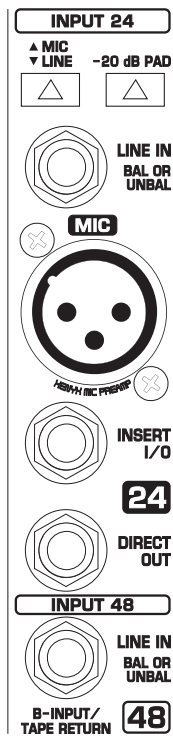
Fig. 7.8: A and B-channel input section
