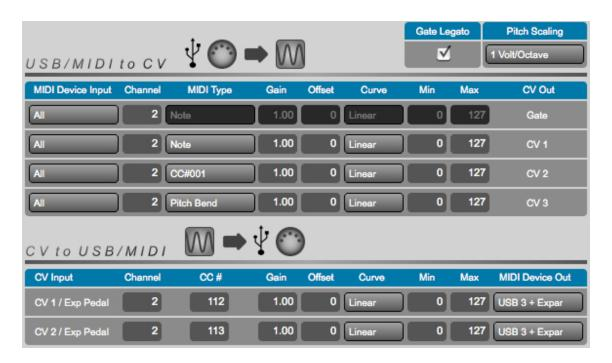
Here you can choose how the QuNexus keys send and receive CV (Control Voltage). QuNexus has 4 possible CV outputs and 2 possible CV inputs (see the CV Manual for the hardware specs).
