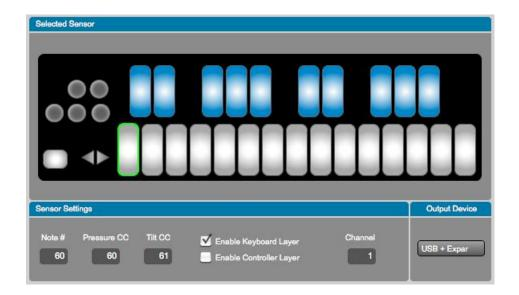
The Controller Layer tab appears next to Keyboard Layer. Here you can assign each key its own additional Note, Pressure CC#, and Tilt CC#. Do this by clicking on any key in the image so that it is highlighted with a green border. Then look below the image at the Sensor Settings.
