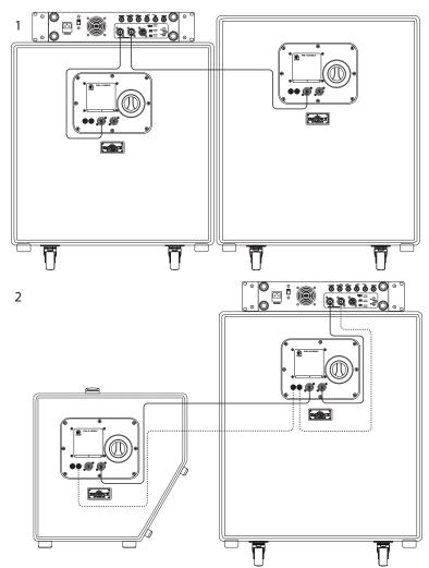
In the first example, a speaker cable with Speakon® ends connects from one speaker output of the amplifier to the speaker input of an Ampeg Pro Neo PN-115HLF cabinet. Additionally, an Ampeg Pro Neo PN-410HLF cabinet is connected from the remaining speaker output of the amplifier to the cabinet's speaker input using speaker cable with Speakon® ends.
