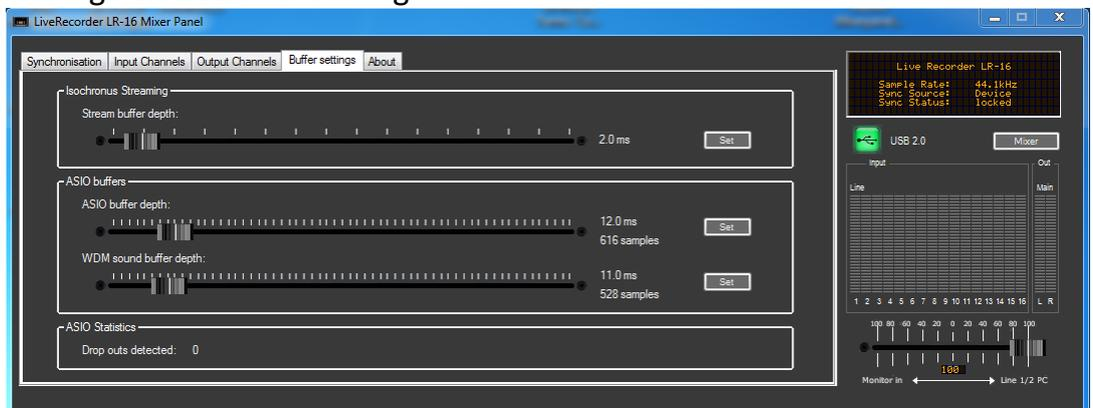
**Isynchronous Streaming Buffer:** Use this slider to adjust the buffer size of the LR-16 drivers.
