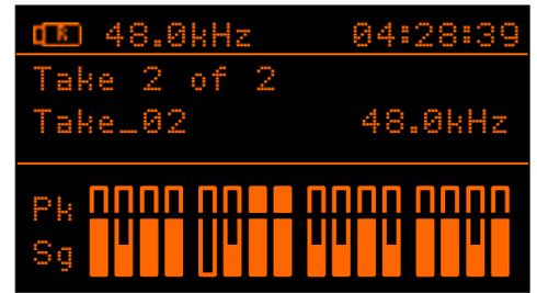
Press the Record **16** button to start the recording. The LR-16 will create a new Take, the record button light will turn red and the 'walking dots' in the display indicate that the recording is running. At the same time the 'Remaining time' indicator in the top right corner will count down the maximum remaining time for this recording. The recording will be stored as 16 separate wave files into the 'Recording/Take\_xx' folder on the USB storage device.
