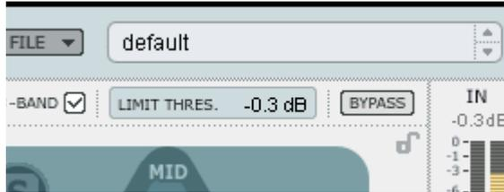
Fabrik C also holds a Limiter. The Limiter is used to prevent overloads occurring at extreme and occasional peaks in the source material, - peaks that may not be caught and attenuated sufficiently in the Compressor. As the Limiter can be used to limit the extreme, the Compressor can be used to apply a much more “musical” and gentle compression.
