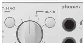
The AUX switch allows you to monitor the signal present on the AUX inputs (rear panel)
