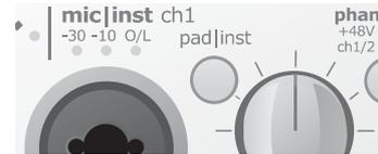
Connecting a Condenser microphone. Konnekt delivers +48v phantom power on the XLR part of the Combo connection for use with condenser microphones. Press “phan” to activate phantom power:
