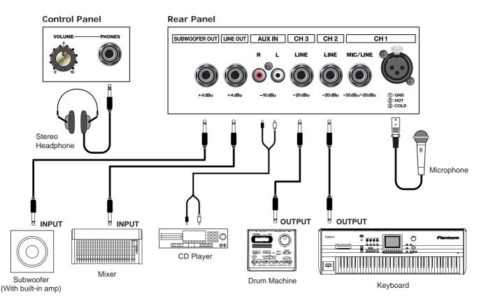
Here is an example of a setup that makes full use of the KC-60's mixer and monitor functions.
