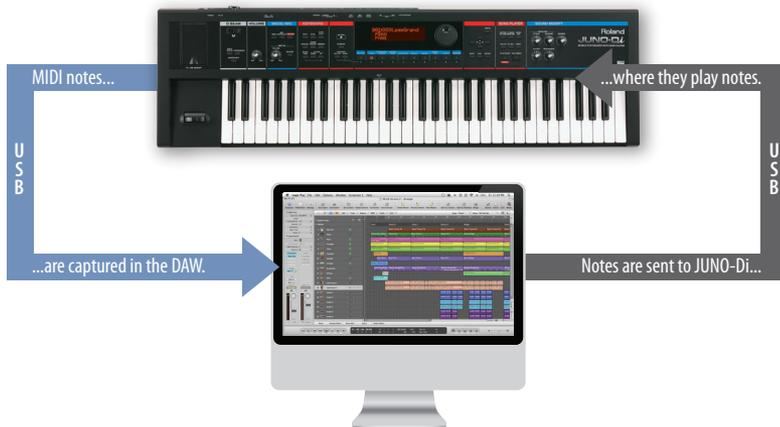
With its light weight and its ability to run on battery power, the JUNO-Di makes an excellent portable MIDI controller for a DAW, especially a laptop DAW. By plugging earbuds or headphones into your computer, you can use a DAW's soft synths; plugging them into the JUNO-Di lets you use JUNO-Di sounds. In a more complex setup, listen to both through an audio interface.
