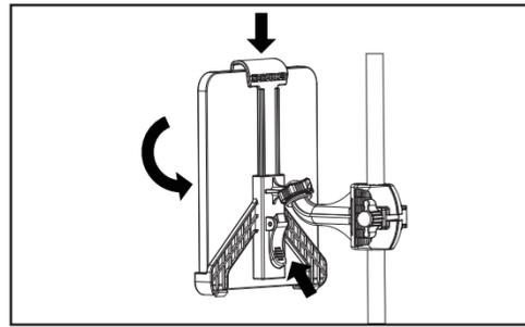
4. Now you can adjust the holder to the best position for your needs. Make sure to loosen the yellow ring every time before adjusting the angle. Likewise, always tighten the ring after adjusting.
