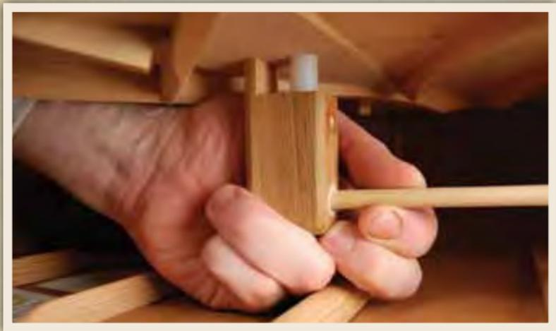
2. Grasp the dowel between your thumb and forefinger, and make sure there is no play along the lateral axis (running the length of the guitar). If there is any movement here, the bridge truss will need to be tightened (see step 4). If there is no movement, move on to step 3.
