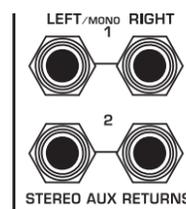
Fig. 2.8: Stereo aux return connectors
