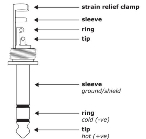
For connection of balanced and unbalanced plugs, ring and sleeve have to be bridged at the stereo plug.
