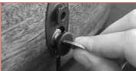
Replacing the battery. With a coin or guitar pick, push in and rotate counter-clockwise 1/8-turn until you hear a click. The above photo indicates how far you should expect to turn.
